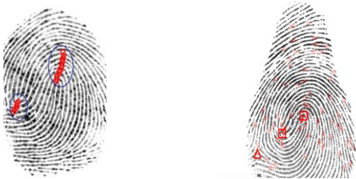
Figure 1. The illustrations of high curvature points (left) and of core point and delta point (right)
